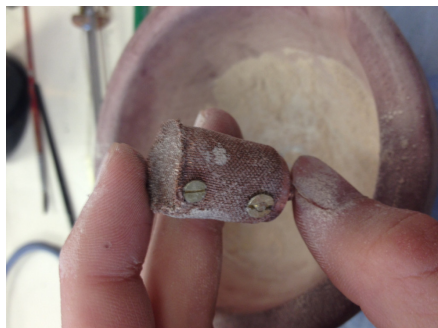
Figure 4: The sorb packed with molecular sieve.
